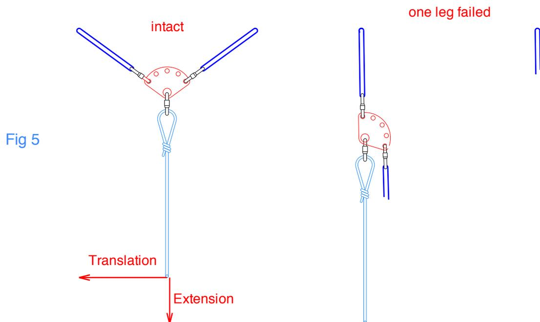
Extension and translation, are a problem because, the sudden shock that occurs, when the remaining leg stops the load from free fall, can, if great enough, cause the entire remaining anchor system to fail. Extension in any anchor system, is to be avoided at all cost. If it exists at all, it must be kept to an absolute minimum.
