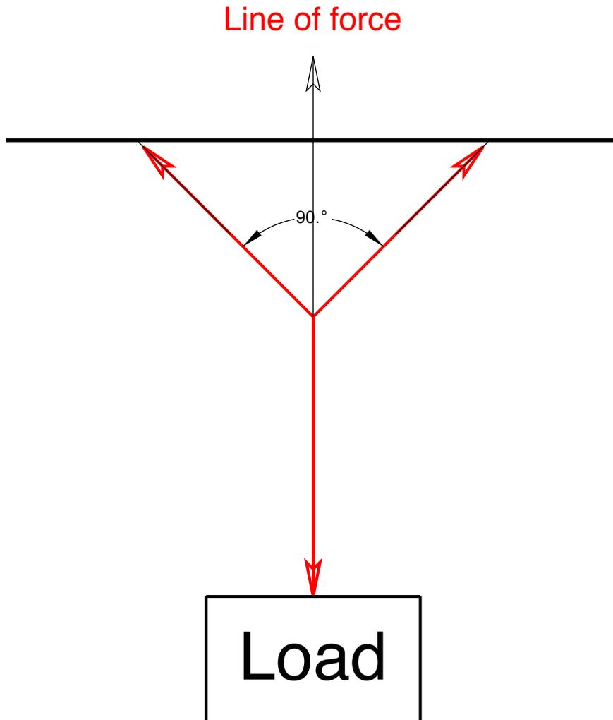
In Fig.1 we can see the line of force bisects the angle formed by the anchor's legs equally. Our goal is to find the actual forces at each anchor point, for a given load.
