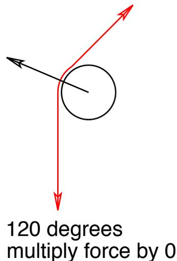
We can use this knowledge to our advantage. We often incorporate c.o.d. pulleys into our systems. So we can diminish the c.o.d. anchor forces by increasing the angle the line runs through the pulley.
